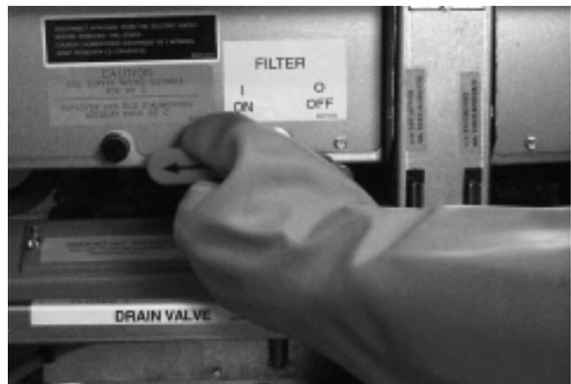
5. The filter pump draws the cooking oil/shortening through the filter and circulates it back up to and through the fryer during a 5-minute process called polishing. Polishing cleans the oil by trapping solid particles in the filter medium.
