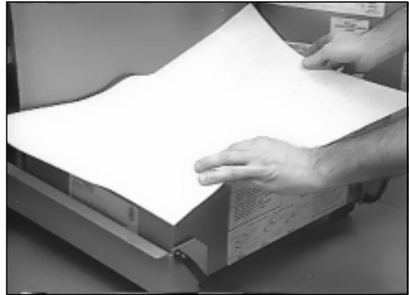
3. Position the hold-down ring over the filter paper and lower the ring into the pan, allowing the paper to fold up around the ring as it is pushed to the bottom of the pan.
