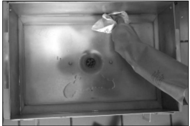
2. After verifying that the metal filter screen is in the bottom of the pan, lay a sheet of filter paper over the top of the pan, overlapping on all sides.
