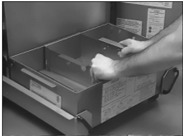
5. Push the filter pan back into the fryer, positioning it all the way to the back of the cabinet. (Some older filter systems have a green HEATER ON indicator, which will light when the assembly is properly positioned.)
