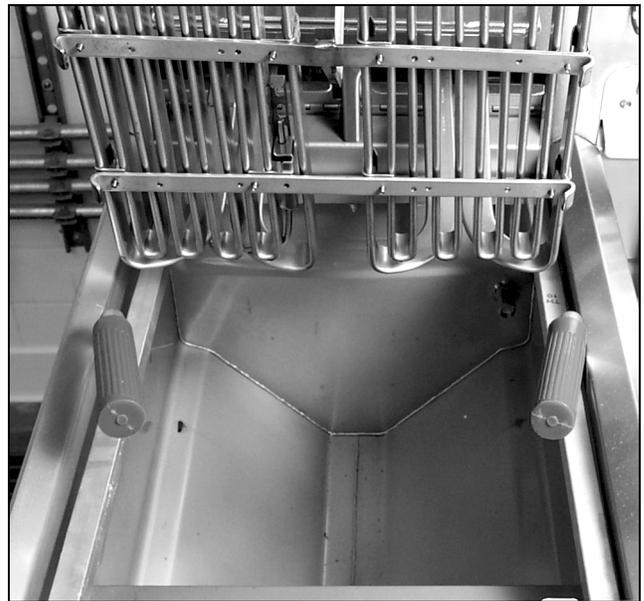
Remove the basket support rack from the frypot, raise the element assembly to the up position, and snap the Power Shower into position.
